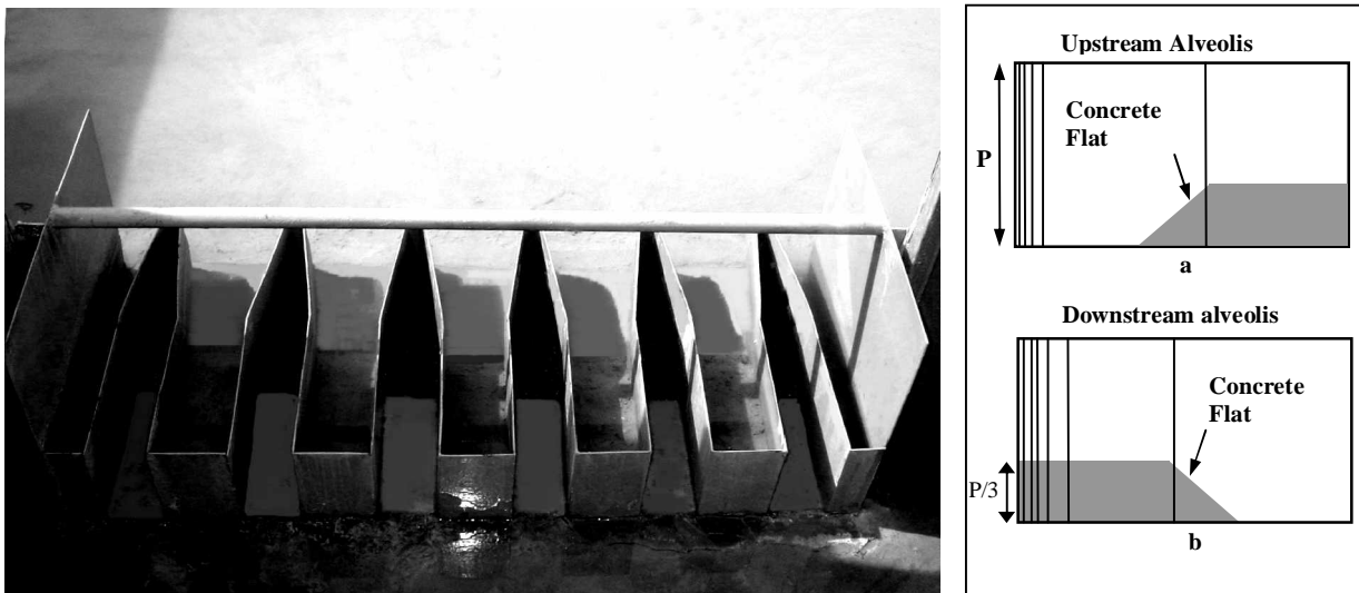
Fig. 3 Labyrinth weir with profiled entrance and partial filling in ordinary concrete inside the inlets and outlets alveoli
